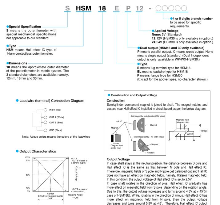
gets around 0.5 V to 4.5V between  $\pm$ 45° in proportion to the rotation angle.
