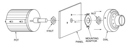
Note: The nut with a mark % is not always used depending on the kind of potentiometer and the thickness of the panel to be mounted.
