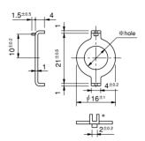
Note: The dimensions of mark  $\mbox{\%}$  are determined by the potentiometer to be mounted.
